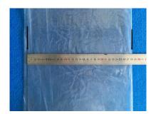
2- Measure the position of all valves from the left end and from the top of the bladder. Take your measure in the valve axis (center of the valve).
